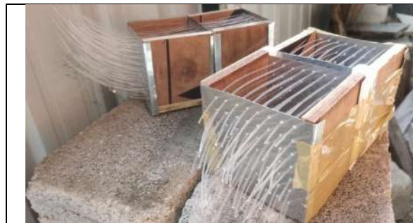
Fig. 1. Placement of fibres in the mould
